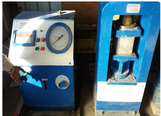
Fig. 2 Testing of Cubes
