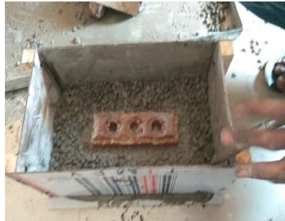
Fig. Plastic strip placed after one layer of concrete in mould
