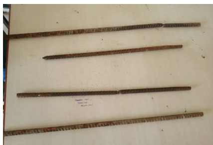
Fig 3(a) Failure of newly manufactured steel bars
