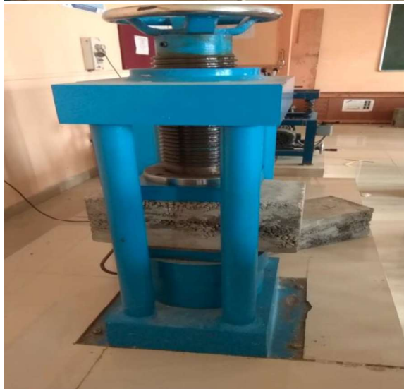
Fig. Testing of block under CTM machine"
