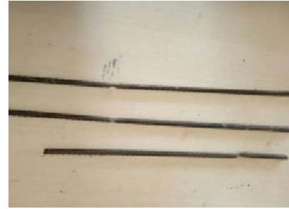
Fig 3(b) Failure of Deteriorated steel bars
