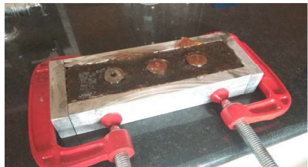
(Fig. Melted PET plastic in the mould )
