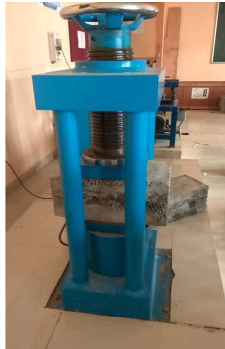
(Fig. Testing of block under CTM machine)
